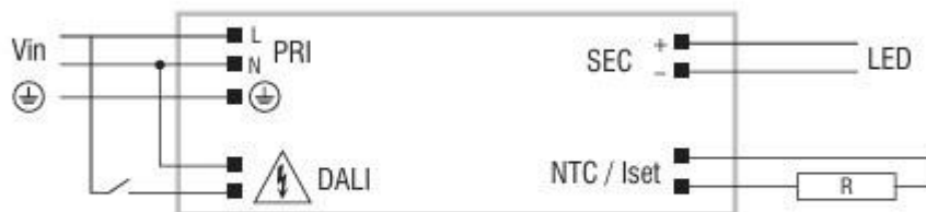
PUSH SWITCH diagram - Collegamento PUSH SWITCH
