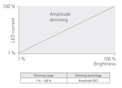
LC27MINI-FD-150-700 LED driver implements amplitude dimming technology across whole dimming range. Amplitude dimming offers the best available technology for dimming the light output in an accurate and flicker-free way to ensure high quality lighting in even the most demanding situations such as camera recording applications. Amplitude dimming technology complies with IEEE 1789-2015 recommendations of current modulation to mitigate health risks to viewers.
