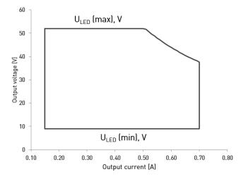
Note: 1) Dimming between 1 % - 100 % possible across the operating window, restricted by the absolute minimum dimming current of 5 mA.
